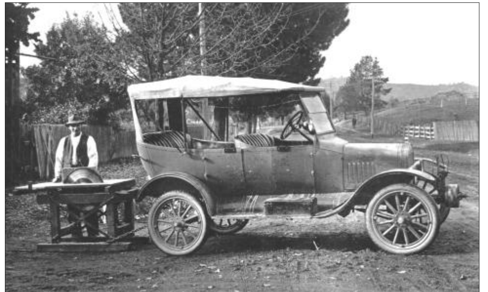
An old car converted to run a circular saw
