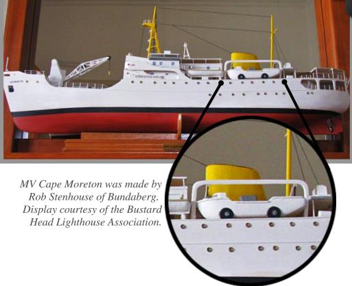
After 1974, a LARC (Lighter Amphibious Resupply Cargo) was carried as deck cargo on the MV Cape Moreton. This was swung outboard and lowered to the water. Supplies were loaded then transported to the lightstation.
