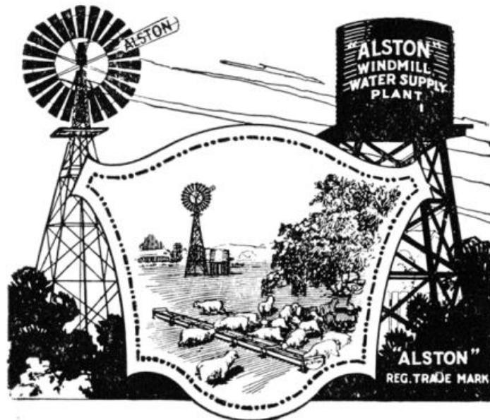
Fitted with Ball Bearings and Machine-cut Gears. All working parts enclosed and running in Oil Bath. Storm-proof and adjustable for speed. Heavy 4-post Steel Angle Towers.
